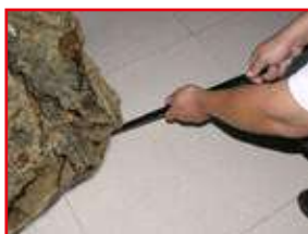
Medium-steel bar for prying, cutting, and digging work
