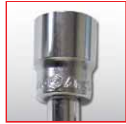
Push to Lock in Standard Position
